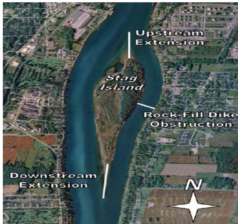
Figure 7. Dikes and Training Structures at Stag Island (IJC, 2012 adapted from Moore, 1933)
