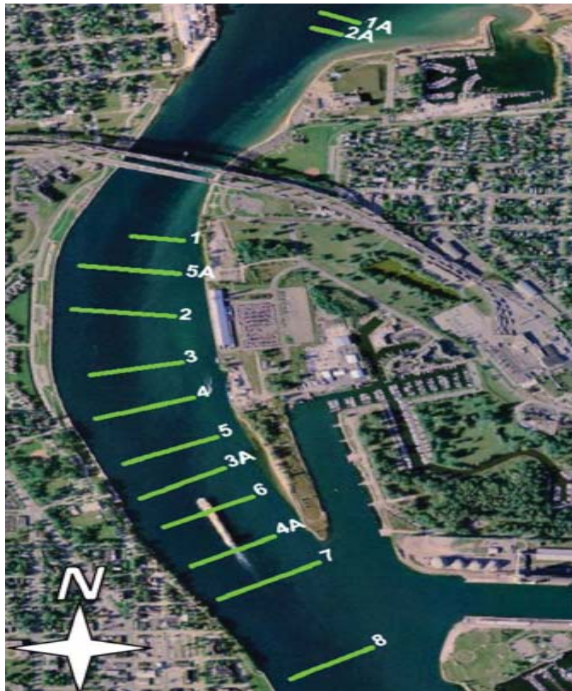
Figure 4. Proposed Submerged Sills (IJC, 2012 adapted from Franco and Glover, 1972)
