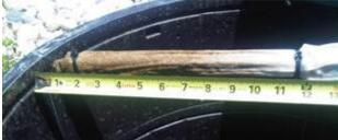
To measure the depth of the sludge layer and the total depth of all of the contents of the tank, slowly lower the stick with the cheesecloth downward into the septic tank until the stick rests on the bottom of the septic tank. When the end of the stick is on the bottom of the tank, take note of where the top of the sludge layer is on the stick.
